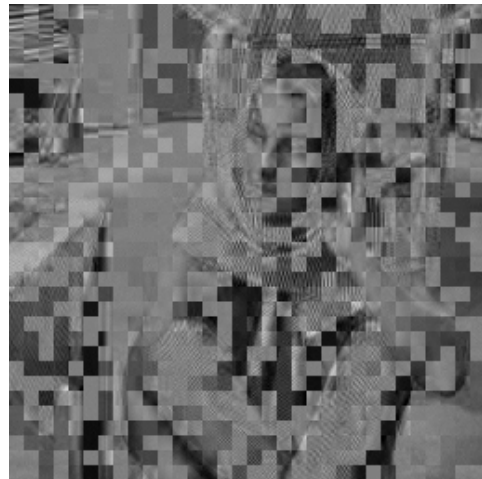
Figure 5. Image quality with the pixel based interleaving in the presence of of random and bursty losses.
