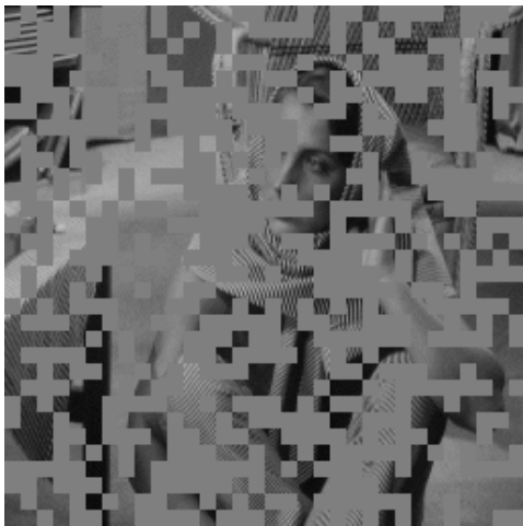
Figure 3. Image quality when entire blocks are interleaved in the transmission sequence in the presence of of random and bursty losses.
