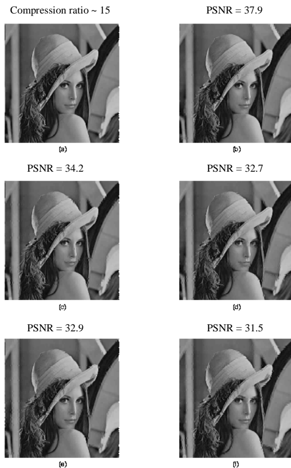
Figure 8: PSNR for different cell loss rates, under 4-MM protection. (a) Represents the original transmitted image, (b)-(f) represent the PSNR under 5%, 10%, 15%, 20%, 25% cell loss rate.
